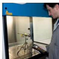
AIR FLOW SPEED TEST
