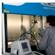
FILTER LEAKAGE TEST
