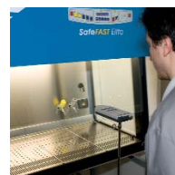
NOISE LEVEL TEST
